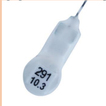
Tags come in different shapes and sizes. Left – Lotek Nanotags; right – CTT Lifetags. Lifetags contain a small solar panel and can therefore last for the length of the bird's life.
